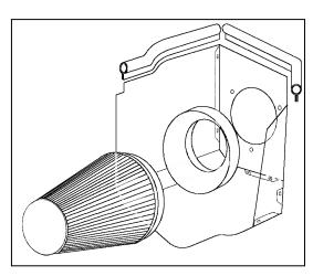
**6.** Using three ½-20x 1/2" button head bolts (#12) and 1/4" flat washers (#13), install the filter adapter (#4) onto the Airaid Cool Air Dam.
