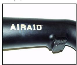
**8.** Using two 8-32x 1/2" button head screws (#15) install the factory **M.A.F.** sensor in the Airaid intake tube (#5) **DO NOT USE THE FACTORY SCREWS!.** (*Note: Sensor must be installed in the direction shown in the picture.*)
