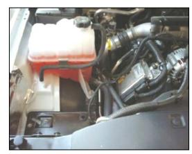
**3.** Remove the factory intake tube assembly from the engine. Rock the factory air box back and forth and remove it from the vehicle. There are only grommets holding it in, no holts
