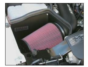
**13.** Install the Airaid filter (#1) onto the filter adapter, and tighten the hose clamp. Install the weather strip (#8) onto the Airaid Cool Air Dam. Reconnect the MAF sensor wiring harness. (Note: Start from one corner and work your way around to insure proper alignment of the weather strip.)
