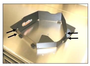
**4.** Assemble the Airaid Quick Fit Panels (#2, #3) using four 6-32x 5/16" screws (#5), #6 flat washers (#6), and 6-32 keps nuts (#7).
