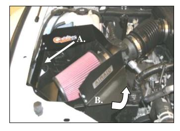
**7. A.)** There are two tabs on the Quick Fit Panel, insert the one closest to the headlight first into the slot on the factory airbox.
