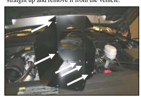
**7.** Assemble the two Cool Air Dam (CAD) panels (#2) and (#3) as shown, using the five 6-32 screws (#10), washers (#11), and nuts (#12).
