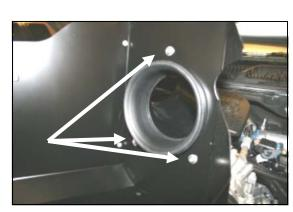
**8.** Install the Airaid intake tube (#4) into the Cool Air Dam using the three 1/4"-20x1/2" button head bolts (#6), and washers (#7) as shown.
