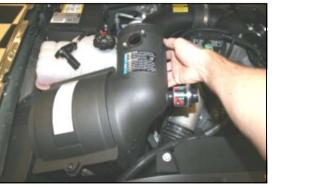
4. Slide the flexible intake tube off of the factory airbox and then rock the airbox back and forth to free it from the mounting grommets, next lift it straight up and remove it from the vehicle.
