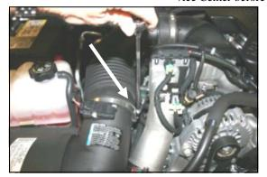
1. <u>Disconnect the negative battery cable.</u> Using a 5/16" socket or flat screwdriver, loosen the hose clamp that holds the factory airbox to the flexible intake tube.
