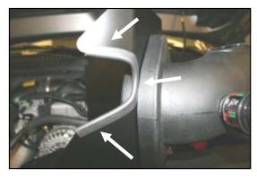
**10.** Install the provided rubber trim (#13) on the **CAD** as shown.
