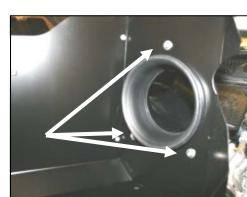
8. Install the Airaid intake tube (#4) into the Cool Air Dam using the three 1/4"-20x1/2" button head bolts (#6), and washers (#7) as shown.
