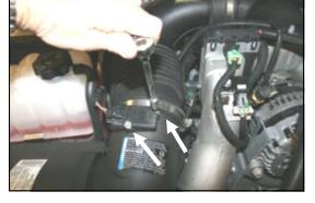
2. Using a #20 Torx bit, remove 2 screws holding the Mass Air Flow sensor to the factory airbox tube.
