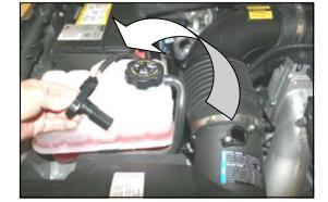
3. Without disconnecting the wiring harness, remove the Mass Air Flow sensor from the factory airbox, and set it aside.
