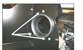
9. Re-install the factory grommet and filter minder removed in step #5 into the Airaid intake
