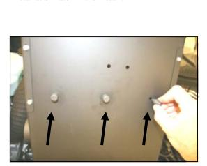
7. Install the three silicone bumpers (#15) into the three holes in the bottom of the Cool Air Dam, as shown.
