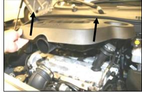
**3.** Remove the factory air filter housing by lifting on the front, and then the rear. There are no bolts holding it down, only 3 rubber grommets.
