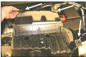
**5.** Remove 3 factory rubber grommets from the factory air cleaner housing.
