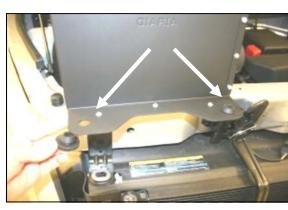
**8.** Install the two large factory grommets removed from the factory air cleaner housing in step #5, into the two holes at the back of the Airaid Cool Air **D**am.
