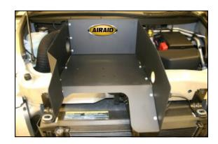
**6.** Assemble the three Cool Air Dam panels (#2, #3, & #4), using 13 screws (#11), washers (#12), and nuts (#13). Apply the Airaid Foil Decal onto
