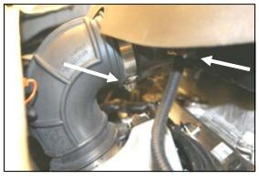
2. Loosen the hose clamp that holds the rubber elbow to the factory air cleaner housing. Next squeeze the tab on the Mass Air Flow sensor wiring connector, and remove the connector from the Mass Air Flow sensor.
