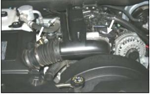
**2.** Using a 5/16" socket or flat blade screwdriver, loosen the hose clamps on both ends of the factory intake tube.
