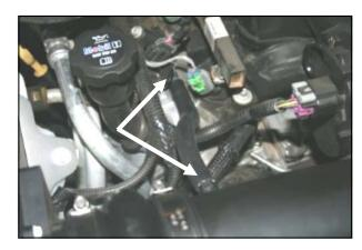
**12.** Slide one end of the 3/8" x 8" breather hose (#16) over the barbed fitting in the Airaid Intake tube. Slide the other end of the breather hose onto the metal tube on the engine.
