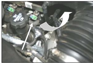
**3.** Slide the factory breather hose off of the metal tube on the engine.
