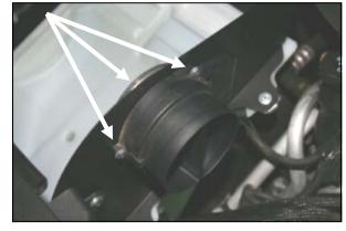
**8.** Mount the **MAF** sensor onto the panel using three 8 -32 x 1/2" button head screws (#11), #8 flat washers (#12), and 8-32 keps nuts (#13). (Note: sensor should be mounted with "flow" arrow on top).
