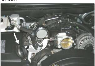
**4.** Loosen the clamp holding the Mass Air Flow (MAF) sensor to the factory airbox lid. Remove the complete factory intake and breather tube. Remove the MAF sensor from the lid (*do not disconnect it*), and then set it aside.
