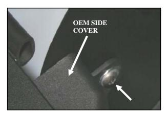
7. <u>6.0 Liter Only:</u> Insert one \(^1\/\_4 - 20 \times 1/2\)" button head bolt (#8) and \(^1/4\)" flat washer (#9) through the hole in the oem side cover, and through the hole in the panel. Secure using one \(^1/4 - 20\) serrated nut (#10).
