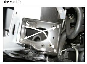
7. Using a 10mm socket, remove four bolts, and then remove the factory airbox mounting plate from the vehicle.
