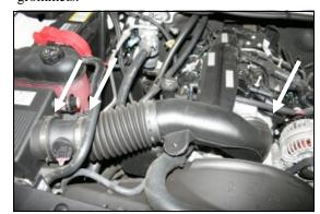
4. Loosen three hose clamps. One at each end of the factory intake tube, and one on the Mass Air Flow sensor (MAF) where it clamps to the factory airbox. Remove the factory intake tube from
