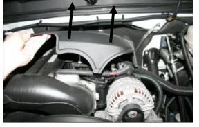
1. <u>Disconnect the negative battery cable.</u> Remove the factory beauty cover by lifting up on the front, and then pulling the cover towards the front of the vehicle. It is only held in place by grommets
