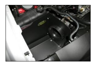
9. Install the Airaid CAD assembly into the vehicle replacing the factory airbox. Secure the CAD using four M6 x 1.25 Hex Bolt (#15), and 1/4" flat washers (#14). Do not over tighten the four bolts.
