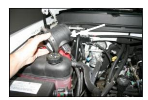
5. Remove, and set aside the MAF (Mass Air Flow) sensor from the factory airbox using caution to retain the factory clamp and seal.
