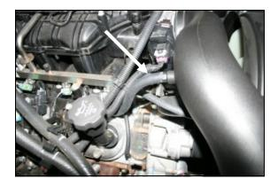
**13.** Install the 3/8" x 8" breather hose (#8) between the 1/4" NPT x 3/8" barbed fitting in the tube, and the factory port on the valve cover.
