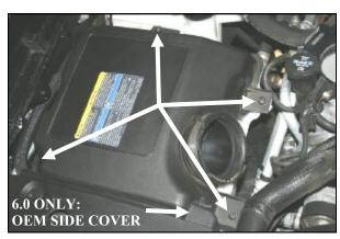
**5.** Loosen the four mounting screws on the factory airbox lid. Remove the factory airbox lid, filter, and resonator as an assembly.
