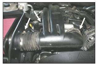
**10.** Reinstall the factory intake tube and tighten the hose clamps. Reconnect the factory crankcase breather tube.
