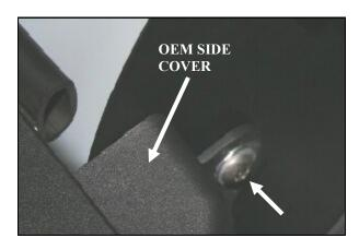
7. <u>6.0 Liter Only:</u> Insert one  $\frac{1}{4}$  - 20 x 1/2" button head bolt (#8) and 1/4" flat washer (#9) through the hole in the factory side cover, and through the hole in the panel. Secure using one  $\frac{1}{4}$  - 20 serrated nut (#10).
