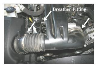
**2.** Using a 5/16" socket or flat blade screwdriver, loosen the hose clamps on both ends of the factory intake tube. Carefully pull the crankcase breather fitting out of the factory intake tube. Remove the factory intake tube from the vehicle.
