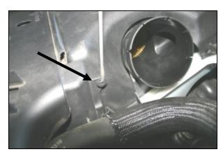
**4.** <u>6.0 Liter Only:</u> Using a flat blade screwdriver, gently pry the plastic retaining clip from the factory side cover. Pull out the center pin, and then remove the clip from the cover.
