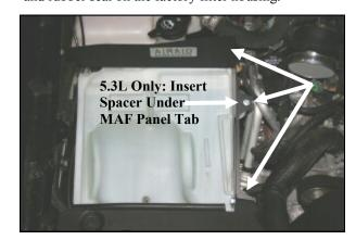
**6.** Mount the **MAF** Panel (#3) onto the airbox base using three M6 x 25mm Hex Bolts (#7), and flat washers (#9).
