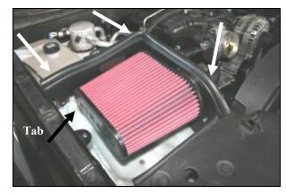
9. Install the Airaid Premium Filter (#1) onto the MAF sensor. Rotate the filter so that the tab contacts the air box base, and then tighten the clamp. Next install the supplied weatherstrip (#3) onto the top of the MAF panel starting at the right fender and work your way towards the radiator.
