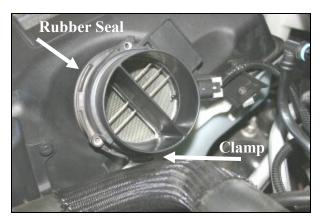
3. Loosen the hose clamp on the Mass Air Flow (MAF) sensor and remove only the sensor from the factory air filter housing without disconnecting the wiring harness. Set it aside for reuse. Leave the clamp and rubber seal on the factory filter housing.
