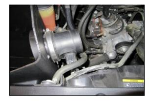
**12.** Reinstall the **MAF** sensor onto the Flter Adapter, and tighten the clamp.
