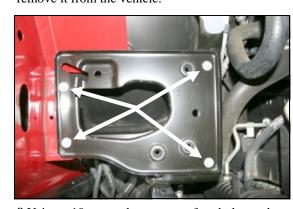
**8.**Using a 10mm socket, remove four bolts, and then remove the factory airbox mounting plate from the vehicle and set aside. Three of these bolts will be reused in step 11.
