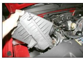
**7.** Rock the factory airbox back and forth to loosen it from the mounting grommets, and remove it from the vehicle.
