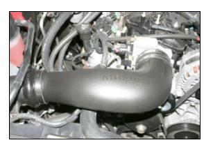
**15.** Install the Airaid Intake Tube into the Hump Hose first, and then onto the throttle body. Adjust for fit, and tighten the hose clamps. Next install the 3/8" x 14" breather hose (#7) between the 1/4" NPT x 3/8" barbed fitting in the tube, and the factory port on the valve cover.
