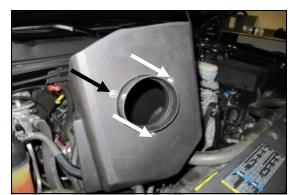
**9.** Install the Filter Adapter (#4) onto the Cold Air Box, or CAB (#3), as shown using the three 1/4 -20 Button Head Bolts (#9) and 1/4" Washers (#10).
