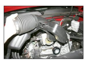
**5.** Slide the factory intake tube off of the **MAF** sensor, rotate it up so that it disengages from the mounting grommet on the intake manifold, and then slide it forward off of the throttle body and remove it from the vehicle.
