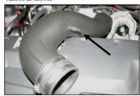
**14.** Install the 1/4" NPT x 3/8" Barb Fitting (#12) into the Airaid Intake Tube as shown. Next install the Urethane Coupler (#6) onto the throttle body end of the tube using two #64 hose clamps (#11). Only tighten the Tube side clamp at this time.
