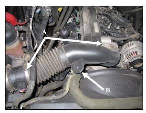
**3.A.**) Loosen the clamps securing the factory intake tube to the throttlebody and the Mass Air Flow Meter, or MAF.
