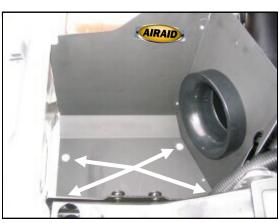
7. Install the Airaid Cool Air Dam assembly in the engine compartment using four M6-1x25 hex bolts (#14) and 1/4" flat washers (#13). Apply the Airaid Foil Decal onto the Panel as shown.
