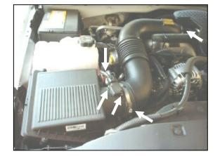
1. <u>Disconnect the negative battery cable.</u> Disconnect the Mass Air Flow (M.A.F.) sensor wiring harness. Using the supplied T-20 Security bit, remove the two screws and the M.A.F. sensor from the tube (save the sensor for reuse). Loosen the hose clamps on each end of the factory intake tube assembly.
