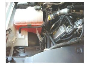
**3.** Remove the factory intake tube assembly from the engine. Rock the factory air box back and forth and remove it from the vehicle. There are only grommets holding it in, no
