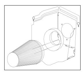
**6.** Using three  $\frac{1}{4}$ -20x 1/2" button head bolts (#12) and 1/4" flat washers (#13), install the filter adapter (#4) onto the Airaid Cool Air Dam.
