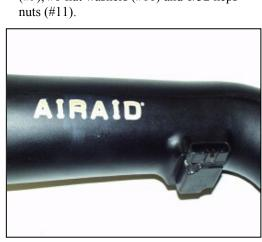
**8.** Using two 8-32x 1/2" button head screws (#15) install the factory M.A.F. sensor in the Airaid intake tube (#5) **DO NOT USE THE** FACTORY SCREWS!. (Note: Sensor must be installed in the direction shown in the picture.)
