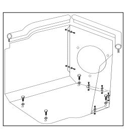
5. Assemble the Airaid Cool Air Dam panels (#2, #3) using five 6-32 x 5/16" screws (#9), #6 flat washers (#10) and 6/32 keps
