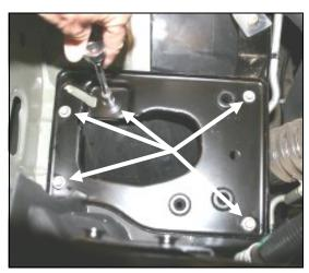
**4.** Using a 10mm socket, remove the five bolts and mounting plate from the engine compart-
