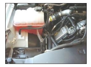
**3.** Remove the factory intake tube assembly from the engine. Rock the factory air box back and forth and remove it from the vehicle. There are only grommets holding it in, no bolts.
