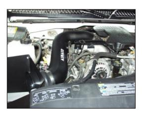
**12.** Install the Airaid intake tube assembly onto the engine. Install the hump hose end onto the filter adapter first and then slip the coupler end of the tube onto the aluminum intake tube. Adjust for fit, and tighten the hose clamps. (Note: There should be a gap in between the Airaid intake tube and the air filter adapter.)
