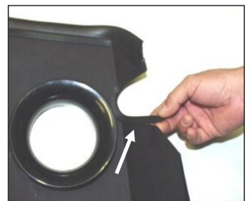
6. Install the 7/4" rubber trim (#12) onto the side of the Airaid Cool Air Dam.
