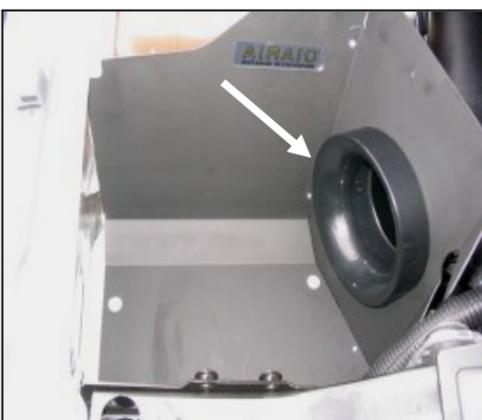
7. Install the filter adapter (#4) using three 1/4-20 x 1/2" button head bolts (#9) and 1/4" flat washers (#10).
