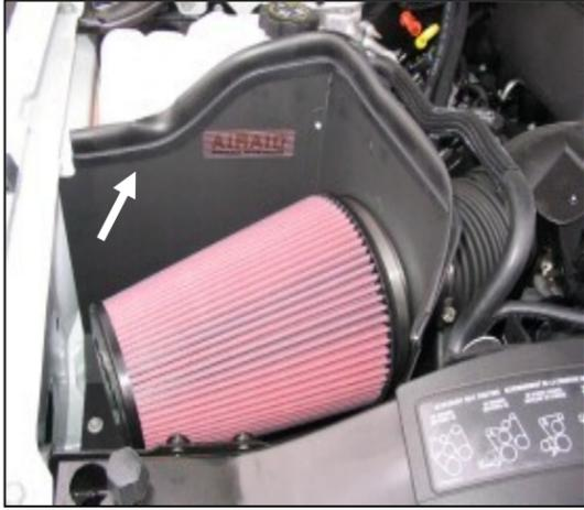
10. Mount the Airaid Premium Filter (#1) onto the filter adapter and tighten the hose clamp. Press the weather strip (#5) along the top edges of the Airaid cool air dam; assure that it is fully seated along the edges. (Hint: *Begin at a corner and work toward the ends.*)
