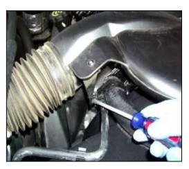
**3.** Using a flat head screwdriver, gently pry the radiator hose bracket from the factory intake tube assembly and remove the intake tube from the vehicle.
