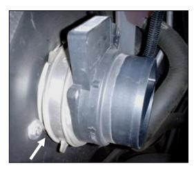
**8.** Slide the factory **MAF** sensor onto the air filter adapter and tighten the hose clamp. (<u>Note</u>: factory clamp / rubber bushing must be in place on the inlet to the MAF sensor.)
