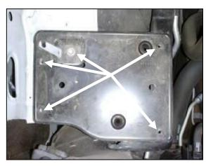
**5.** Using a 10mm socket, remove the five bolts that secure the factory air filter housing platform and remove it.
