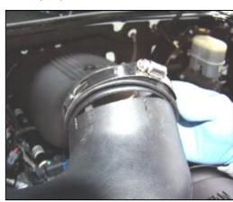
**9.** Install the GM coupler (#7) onto the throttle body side of the Airaid Intake Tube (#5).
