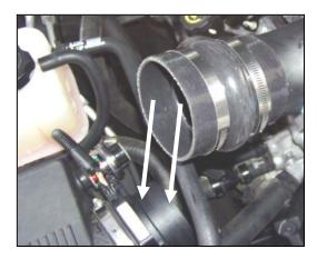
**10.** Install the urethane hump hose (#6) onto the Airaid Intake Tube (#5) and the **MAF** sensor with two #60 hose clamps (#15). Install the tube assembly onto the engine. (*Hint: slide the hump hose all the way onto the end of the tube*)
