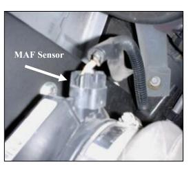
**2.** Disconnect the **MAF** sensor wiring harness and remove the sensor from the factory intake tube.
