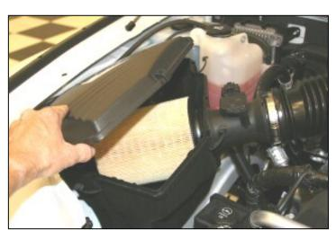
**2.** Remove the lid by lifting, and sliding it out of the tabs on the side of the airbox.
