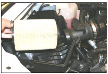
**3.** Remove the factory air filter from the airbox. Do not remove the factory airbox base. The factory base is required to mount the Airaid Quick Fit Panel.
