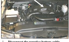
1. <u>Disconnect the negative battery cable.</u> Using a 5/16" socket, remove one bolt on the top of the beauty cover. Set the bolt and the cover aside for re-installation later.
