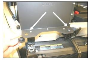
**8.** Install the two large factory grommets removed from the factory air cleaner housing in step #5, into the two holes at the back of the Airaid Cool Air **D**am.
