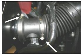
**9.** Re-install the Mass Air Flow sensor and coupler onto the air filter adapter (#4), as shown and tighten the hose clamp. Next re-connect the factory intake tube to the Mass Air Flow sensor, and tighten the hose clamp.
