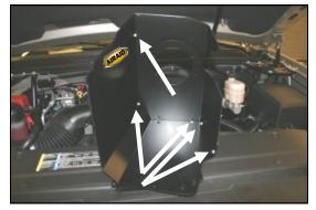
6. Assemble the two Cool Air Dam panels (#2)
