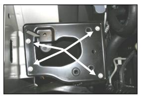
**5.** Remove 4 bolts, and remove the factory air-
