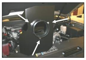
**7.** Install the filter adapter (#4) into the **CAD** using three button head bolts (#6), and washers (#7).
