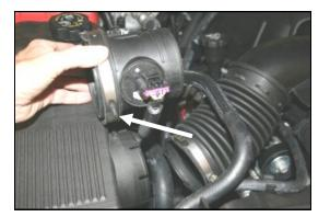
2. Remove the Mass Air Flow sensor from between the factory intake tube and the factory air box. Use caution to retain the rubber coupler on the Mass Air Flow sensor.
