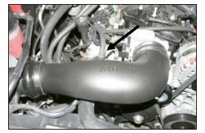
14. Install the Airaid Intake Tube into the hump hose first, and then onto the throttle body. Adjust it for fit, and tighten the hose clamps. Next install the 3/8" x 14" breather hose (#8) between the 1/4" NPT x 3/8" barbed fitting in the tube, and the factory port on the valve cover.
