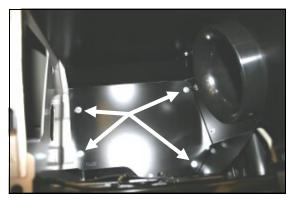
10. Install the Airaid CAD into the vehicle replacing the factory airbox. Secure the CAD using four M6 x 1.25 Hex Bolt (#15), and  $1/4^{\circ}$  flat washers (#14). Do not over tighten the four bolts.
