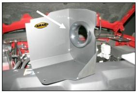
**9.** Assemble the Cool Air Dam panels (CAD) (#2 & #3) using five 6-32 x 5/16" screws (#10), #6 flat washers (#11), and 6-32 keps nuts (#12). Next install the air filter adapter (#5) into the panels as shown using three  $1/4 - 20 \times 1/2$ " button head bolts (#13), and 1/4" flat washers (#14). Apply the Airaid Decal as shown.
