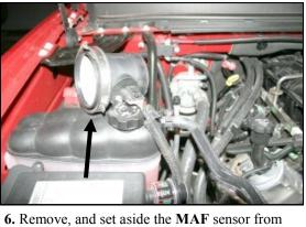
4. Loosen three hose clamps. One at each end of the factory intake tube, and one on the Mass Air Flow sensor (MAF) where it clamps to the factory airbox.
