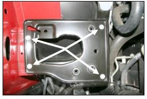
**8.**Using a 10mm socket, remove four bolts, and then remove the factory airbox mounting plate from the vehicle.
