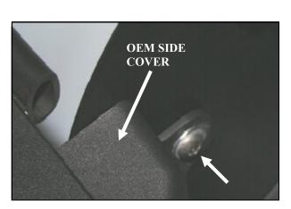
7. <u>6.0 Liter Only:</u> Insert one  $\frac{1}{4}$  - 20 x 1/2" button head bolt (#8) and 1/4" flat washer (#9) through the hole in the oem side cover, and through the hole in the panel. Secure using one  $\frac{1}{4}$  - 20 serrated nut (#10).
