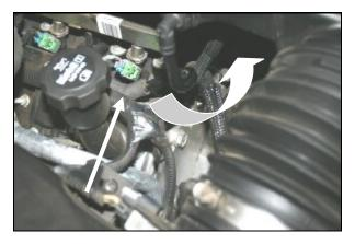
**3.** Slide the factory breather hose off of the metal tube on the engine.
