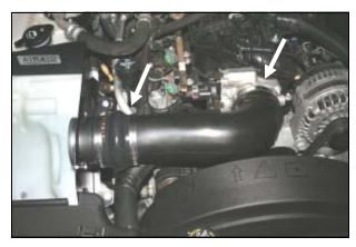
11. Insert the Airaid Intake Tube (#2) into the hump hose first. Then, insert the throttle body end of the tube into the coupler. Adjust for fit, and tighten the clamps.
