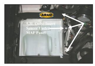
**6.** Mount the MAF Panel (#3) onto the airbox base using three M6 x 25mm Hex Bolts (#7), and ½" flat washers (#9). Apply the Airaid Foil Decal onto the Panel as shown.
