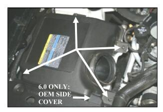
**5.** <u>**6.0** Liter Only:</u> Using a flat blade screwdriver, gently pry the plastic retaining clip from the oem side cover.
