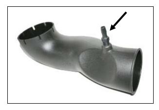
**10.** Insert one  $\frac{1}{4}$ " NPT x  $\frac{3}{8}$ " barbed fitting (#15) into the Airaid Intake Tube (#2).
