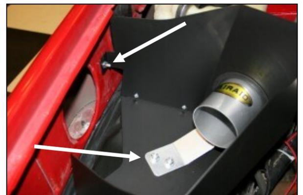
4. Insert the Airaid intake tube (#5) thru the hole in the MAF panel and then rotate it clockwise so that the holes in the bracket on the tube line up with the two holes in the bottom panel. Apply the Airaid Decal onto the Intake Tube as shown.
