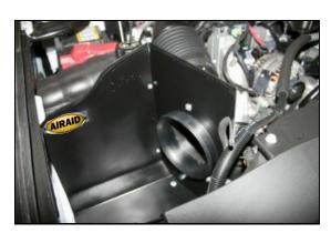
**8.** Install the Cool Air Dam into the vehicle where you removed the factory mounting plate in step #4, using the four supplied M6-1x25 bolts (#9), and flat washers (#7).
