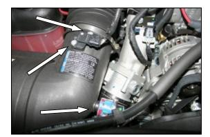
2. With a #20 Torx bit, remove 2 screws holding the Mass Air Flow sensor to the factory airbox tube. Remove the MAF and set it aside. Remove the factory filter minder and grommet from the factory airbox. Save them for later use in step #10.
