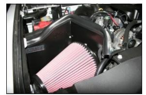
11. Install the Airaid Premium Filter (#1) onto the Airaid intake tube (#4), and tighten the hose clamp. Now install the provided weather strip (#5) on the top of the CAD. For ease of installation, start near the fender and work your way towards the radiator.
