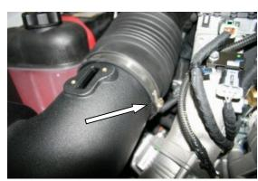
**9.** Reconnect the factory intake tube to the Airaid Intake Tube, and tighten the hose clamp.
