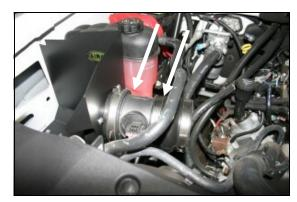
10. Reinstall the MAF sensor onto the filter adapter, and tighten the clamp. Next install the urethane hump hose (#6) onto the MAF with the two #64 hose clamps (#16). Tighten only the hose clamp that secures it to the MAF.
