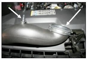
11. Install the 1/4" NPT x 3/8" Barb Fitting (#17) into the Airaid Intake Tube as shown. Next install the supplied coupler and hose clamp (#7) onto the throttle body end of the tube. Leave the clamp loose for now.
