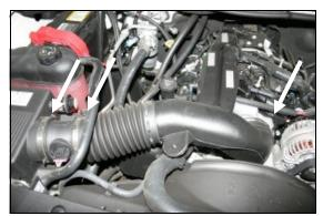
**4.** Loosen three hose clamps. One at each end of the factory intake tube, and one on the Mass Air Flow sensor (MAF) where it clamps to the factory airbox. Remove the factory intake tube from the vehicle.
