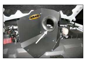
**8.** Assemble the Cool Air Dam panels (CAD) (#2 & #3) using five 6-32 x 5/16" screws (#10), #6 flat washers (#11), and 6-32 keps nuts (#12). Next install the air filter adapter (#5) into the panels as shown using three 1/4 - 20 x 1/2" button head bolts (#13), and 1/4" flat washers (#14). Apply the Airaid Foil Decal onto the Panel as shown.
