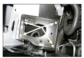
**7.** Using a 10mm socket, remove four bolts, and then remove the factory airbox mounting plate from the vehicle.
