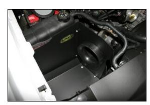
9. Install the Airaid **CAD** assembly into the vehicle replacing the factory airbox. Secure the **CAD** using four M6 x 1.25 Hex Bolt (#15), and 1/4" flat washers (#14). Do not over tighten the four bolts.
