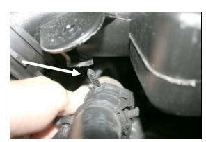
**3.** Separate the factory intake tube from the plastic clamp that secures the radiator hose to the tube. A firm downward push will usually do it.
