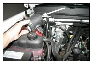
**5.** Remove, and set aside the **MAF** (**Mass Air** Flow) sensor from the factory airbox using caution to retain the factory clamp and seal.
