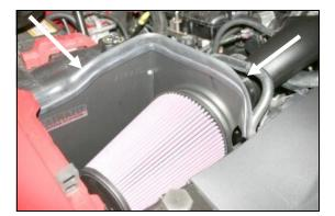
13. Install the Airaid Premium Filter (#1) onto the air filter adapter, and tighten the hose clamp. Next install the provided weather strip (#9) onto the top of the CAD. For ease of install, start at the inner fender, and work your way towards the radiator. Reinstall the beauty cover.
