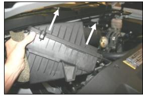
6. Rock the factory airbox back and forth to loosen it from the mounting grommets, and remove it from the vehicle.
