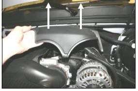
1. Disconnect the negative battery cable. Remove the factory beauty cover by lifting up on the front, and then pulling the cover towards the front of the vehicle. It is only held in place by
