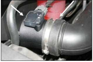
**8.** Reinstall the **MAF** sensor onto the filter adapter using two  $8-32 \times 5/8$ " button head screws (#9).
