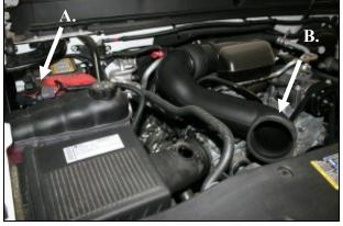
**2.** A.) Without disconnecting the wiring harness, remove the **MAF** sensor from the airbox lid and swing it back out of the work area. B.) Now disconnect the factory air intake tube from the airbox lid, and move it out of the work area. **V-8 Models:** Remove the factory intake tube for ease of install.
