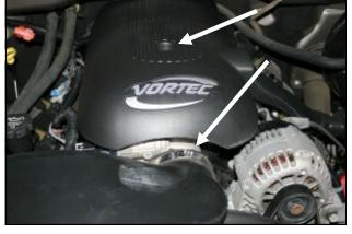
1. Disconnect the negative battery cable. Loosen the bolt that secures the beauty cover to the engine and remove it and the cover from the vehicle. Loosen the hose clamp that secures the factory air intake tube to the throttlebody.
