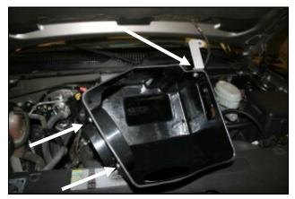
6. Install the filter adapter (#4) into the Cool Air Box (#3) as shown using three 1/4" Button head bolts (#8) and three 1/4" flat washers (#11). Next, fasten the brack
