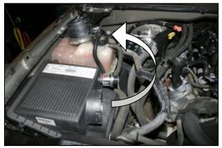
**3.** Remove the factory intake tube from the vehicle. Next, remove the MAF sensor and coupler from the factory airbox and set them out of the way without disconnecting the wiring harness.
