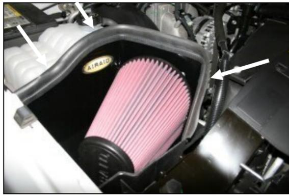
8. The Airaid Premium filter (#1) is a very tight fit in the CAB. For ease of installation, hold the filter in your right hand, and guide the bottom of the filter past the flange of the tube with your left hand inside of the CAB. **It will fit!** Tighten the hose clamp. Next install the weather strip (#5) on top of the CAB, starting at the fender and working your way towards the radiator.
