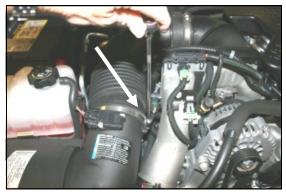
1. **Disconnect the negative battery cable.** Using a 5/16" socket or flat screwdriver, loosen the hose clamp that holds the factory airbox to the flexible intake tube.
