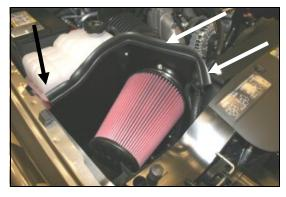
**13.** Install the Airaid Premium Filter (#1) onto the Airaid intake tube (#4), and tighten the hose clamp. Now install the provided weather strip (#5) on the top of the **CAD**. For ease of installation, start near the fender and work your way towards the radiator.
