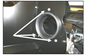
**8.** Install the Airaid intake tube (#4) into the Cool Air Dam using the three 1/4"-20x1/2" button head bolts (#6), and washers (#7) as shown.
