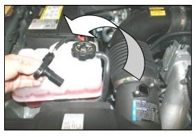
**3.** Without disconnecting the wiring harness, remove the Mass Air Flow sensor from the factory airbox, and set it aside.
