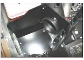
11. Install the assembled CAD into the vehicle where you removed the factory mounting plate in step #6. Use four bolts (#9), and washers (#7) to secure the CAD. Do not over tighten the bolts.
