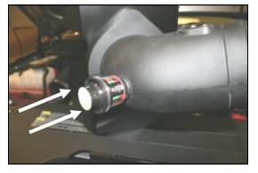
**9.** Re-install the factory grommet and filter minder removed in step #5 into the Airaid intake tube.
