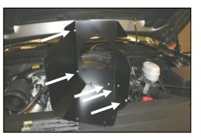
7. Assemble the two Cool Air Dam panels (#2) and (#3) as shown, using the five 6-32 screws (#10), washers (#11), and nuts (#12)
