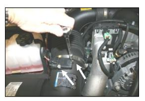
**2.** Using a #20 Torx bit, remove 2 screws holding the **M**ass **A**ir Flow sensor to the factory airbox tube.
