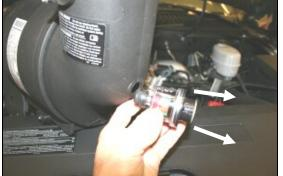
**4.** Slide the flexible intake tube off of the factory airbox and then rock the airbox back and forth to free it from the mounting grommets, next lift it straight up and remove it from the vehicle.
