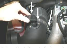
12. Re-position the factory intake tube onto the Airaid tube, and tighten the hose clamp. Next reinstall the Mass Air Flow sensor into the Airaid tube <u>using the two provided Button Head</u> <u>screws (#8)</u>. <u>Do not use the factory screws!</u> Do not over tighten!
