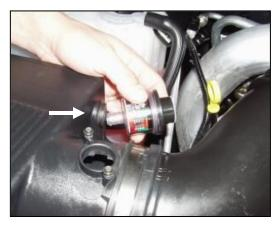
**2.** Remove the factory filter minder and grommet.
