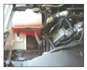
**3.** Remove the factory intake tube assembly from the engine. Rock the factory air box back and forth and remove it from the vehicle. There are only grommets holding it in, no bolts.
