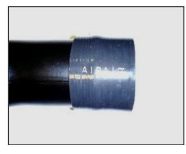
**11.** Install the urethane coupler (#7) and two #60 hose clamps (#17) onto the small end of the Airaid intake tube. (*Note: Leave hose clamps loose until final assembly.*)
