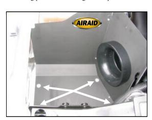
7. Install the Airaid Cool Air Dam assembly in the engine compartment using four M6-1x25 hex bolts (#14) and 1/4" flat washers (#13). Apply the Airaid Foil Decal onto the Panel as shown.
