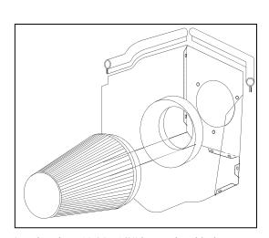
**6.** Using three  $\frac{1}{4}$ -20x 1/2" button head bolts (#12) and 1/4" flat washers (#13), install the filter adapter (#4) onto the Airaid Cool Air Dam.
