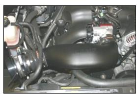
**12.** Install the Modular Intake Tube into the hump hose first, and then into the throttle body. Adjust for fit, and tighten all four hose clamps. Re-insert the plastic piece from step #3 into the hole on the bottom of the MIT.
