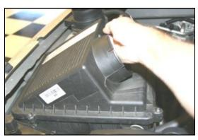
**5.** Grab the factory airbox and rock it back and forth, and remove it from the vehicle. It is only held in by grommets, no bolts.
