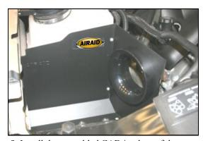
**9.** Install the assembled CAD in place of the factory airbox using four bolts (#11) and washers (#10). Do not over tighten the bolts.
