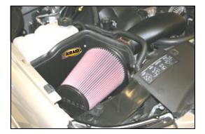
13. Install the Airaid Premium Filter (#1) onto the filter adapter (#5), and tighten the hose clamp. Next install the weather strip (#8) onto the top of the CAD as shown. For ease of installation start at the fender, and work towards the radiator.
