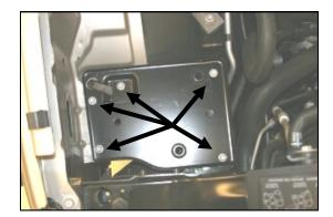
**6.** Remove 5 bolts and remove the factory airbox mounting plate.
