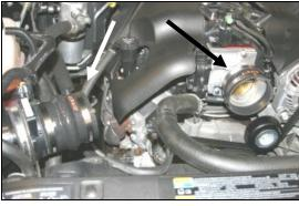
11. Install the urethane hump hose (#6) on the Mass Air Flow sensor with two #60 hose clamps (#15). Next install the coupler (#7) on the throttle body with two #64 hose clamps (#16).
