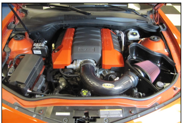
20. Reinstall the engine cover and oil fill cap. Double check your work! Make sure there is no foreign material in the intake path. Make sure all clamps, hoses, bolts, and screws are tight. Reconnect the negative battery cable!
