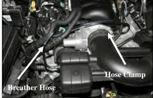
2. Pull the crankcase breather hose out of the air intake tube using a firm tug. An O-ring is all that keeps it attached to the tube. Push the small tab on the hard plastic crankcase breather hose on top of the passenger side rocker cover to release it from the steel breather line. Remove it from the vehicle. Next loosen the hose clamp that secures the air intake tube to the throttle body.
