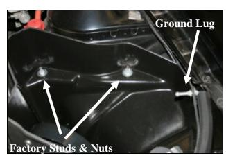
13. Install the Airaid CAB assembly into the vehicle locating the factory grommets over the factory studs. Reinstall the factory nuts from step #3 onto the studs. Reinstall the factory ground lug thru the CAB and thru the side bracket using one flat washer (#12), and one 6mm flange nut (#15). Refer to the line drawing on the first page for reference.
