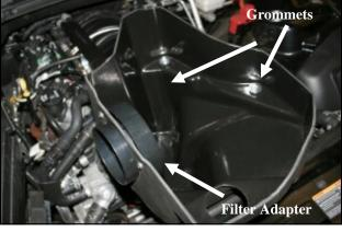
**8.** Reinstall the two steel sleeves and grommets into the Airaid Cold Air Box (CAB) (#3). Next install the filter adapter (#4) into the CAB as shown using three 1/4-20 button head bolts (#9), and 1/4" flat washers (#11). Refer to the line drawing above for details.
