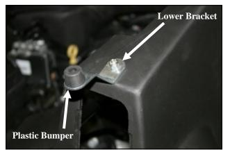
**9.** Turn the CAB upside down and mount the lower bracket (#26) to the bottom of the CAD using one 1/4-20x3/4" hex bolt (#10), 1/4" flat washer (#11), and 1/4" Nylock nut (#13) as shown. Next using one 8-32x5/8" button head screw (#17), and one #8 Kep nut (#18), attach the plastic bumper (#19) to the bracket as shown.
