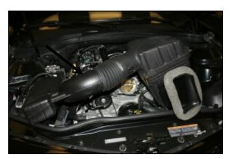
**4.** Lift the complete air intake assembly straight up and out of the vehicle.
