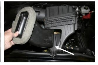
**6.** Squeeze the sides of the factory intake scoop and remove it from the factory airbox. It will be reused in step #10.
