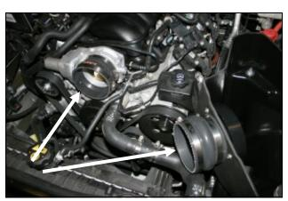
**14.** Install the hump hose (#6) onto the filter adapter using two #64 hose clamps (#23). Next install the reducing coupler (#5) with one #60 hose clamp (#22) on the throttlebody and one #68 hose clamp (#24) on the large end.
