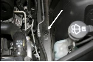
**5.** Use caution not to loose the factory grommet when you remove the air intake assembly. It will be needed if you ever want to reinstall the factory intake assembly.
