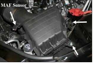
**3.** Using a deep 10mm socket, remove and save the two nuts that secure the factory airbox to the fender well. Using a 9/32" wrench or a #20 Torx bit, remove the two screws that secure the Mass Air Flow (MAF) sensor into the air intake tube. Without disconnecting the MAF, carefully remove it from the tube and set it out of the way on top of the engine.
