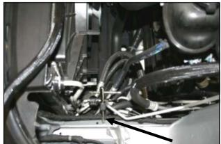
**5.** Locate the pre existing hole in the chassis and tap it for a 1/4-20 bolt. Use a 1/4-20 NC tap with anti-seize lube or equivalent, and follow the 1/4 turn forward, 1/2 turn back rule. This will ensure that clean threads will be cut into the hardened steel. **NOTE:** If your vehicle has a grounding cable bolted to the chassis in this location, you are omit this step.
