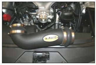
**10.** Install the Reducer Coupler (#8)onto the 90 deg. Bend of the Airaid Intake Tube (#2) and place and the Hump Hose on the opposite end as shown. Secure the couplers to the Intake Tube using the two #64 clamps (#22). Place the #48 clamp(#24) on the reducing coupler and the remaining #52 clamp(#23) on the Hump Hose.
