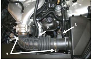
2. A) Loosen the hose clamps on the factory intake tube
