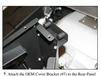
a shown using the remaining two sets of 6-32 hardware
