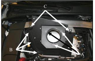
8. A) Install the Filter Adapter onto the MAF panel using three 1/4-20 Button Head screws (#17) and 1/4" Flat washers (#18). B) Attach the Weather Strip (# 11) to the curved edge of the MAF Panel. C) Insert the 5/8" hose anchors (#29) into the two horizontal tab holes on the MAF panel
