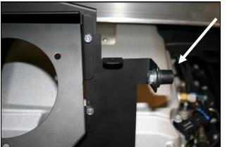
7. Attach the 5/8" Well Nut (#23) to the vertical MAF Panel tab as shown using the 5/16 Hex Bolt (#21) and the 5/16" flat washer (#22).
