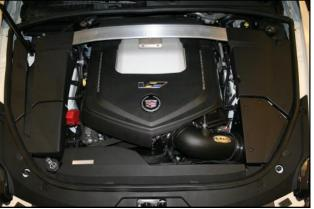
14. Reinstall the Factory engine and shock tower covers.
