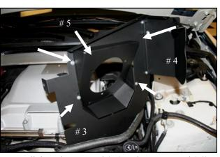
5. Install the Adapter Panel (#5) to the MAF Panel (#3)
