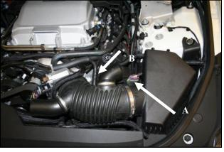
2. A) Disconnect the Mass Air Flow (MAF) sensor. B) Disconnect the PCV breather line by depressing the 2 Grey buttons in the fitting and pulling. Loosen the clamps securing the intake tube to the throttle body and airbox and remove the factory intake tube.
