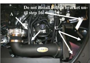
**14. A)** Replace the factory breather line on the valve cover with the 26" Airaid Breather Hose(#12). **B)** Secure the breather hose to the intake tube nipple using the black Speed Clamp (#32).**C)** Slide the Edge Clip Cable Ties (#31) about 6" apart along the fender pinch weld and return the coolant line to it's original location. Secure the coolant line using the cable ties and trim off excess.
