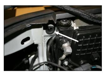
**4.** Use caution not to loose the factory core support grommet while removing the air box assembly. It will be needed in step 13.
