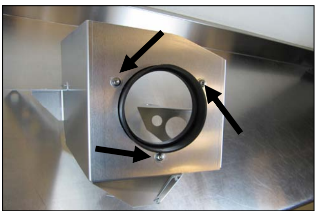
6. Install the Filter Adapter onto the Air Dam as shown using the three Button Head Screws and Flat washers.
