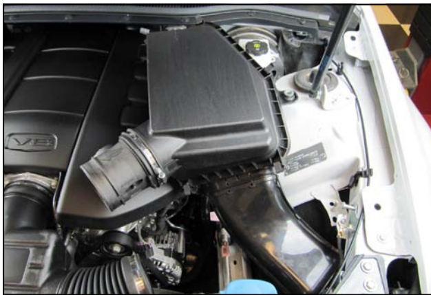
4. Separate the intake tube from the Mass Air Flow sensor and remove the entire air box assembly from the vehicle.
