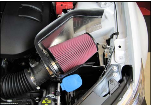
15. Install the Weatherstrip onto the top edge of the Air Dam with the contour rolling away from the Filter.
