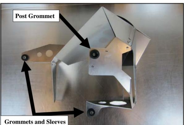
**7. Transfer the OEM grommets and steel sleeves from the factory air box, into the Air Dam assembly as shown. The grommets and steel sleeves are located on the upper half of the box and the post grommet in the lower half.**
