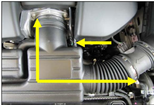
**2. Loosen the intake tube clamps. Disconnect the Valve cover breather and remove the factory intake tube.**
