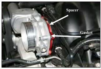
**4.** Install the Airaid Spacer between the throttle body and the intake manifold with the supplied gasket next to the throttle body as shown. \*Note: Airaid spacer must be installed with bore protruding into intake manifold away from throttle body. Incorrect installation will hinder performance. Reference picture below for spacer orientation.
