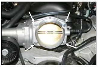
**5.** Install the provided bolts and washers thru the throttle body, gasket, and Airaid Spacer and tighten to the manufacturer's specifications.
