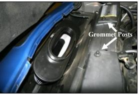
11. Set the Airaid Premium Filter into the area in front of the radiator. It will be mounted in step # 15
