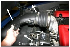
**3.** Lift up on the factory intake tube assembly to disengage the grommets from the two grommet posts and throttle body. Remove the assembly from the vehicle.
