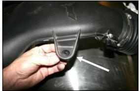
**4.** Remove the two factory grommets from the factory intake tube and set them aside for reuse in step #8.
