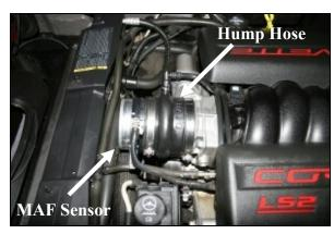
9. Install the hump hose with the #64 hose clamp on the throttlebody. Adjust it so that the breather hose aligns with the barbed fitting, and reconnect the breather. Tighten the hose clamp on the throttlebody. Reinstall the MAF sensor into the hump hose making sure the "Flow" arrow is pointing towards the engine. Tighten the remaining hose clamp.
