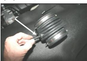
**3.** Remove the barbed fitting from the factory coupler. It will be reused in step #4.
