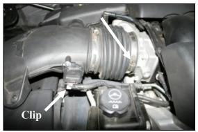
1. <u>Disconnect negative battery cable.</u> Remove the grey security clip on the bottom of the Mass Air Flow sensor wiring connector. Next squeeze the tab on the bottom of the connector. and disconnect the wiring harness from the sensor. Now loosen the hose clamp holding the tube to the throttle body.
