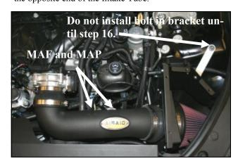
**13.** Install the Airaid Intake Tube assembly onto the filter adapter first, and then onto the throttle body. Adjust for fit, and tighten all the hose clamps. Next, reconnect the **MAF** and **MAP** sensors. Apply the Airaid Bubble Decal onto the Intake Tube as shown.
