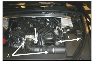
2. A) Loosen the hose clamps on the factory intake tube. B) Disconnect the breather line and remove the factory intake tube . C) Disconnect the Mass Air Flow and MAP sensors.
