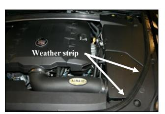
15. A) Install the 11" Weather Strip (#11) onto the curved edge of the top cover (#6) and install the top cover onto the Airaid filter box using the four 1/4-20 Black screws.(#22). B) Line up the intake bracket with the fender bolt hole, and secure the assembly using the factory bolt. Reinstall the Factory engine and shock tower covers .Note: These steps must be performed in order to avoid difficulty with bolt hole alignment.
