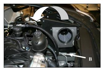
**12. A)** Lower the Airaid Performance Air box assembly into the engine cavity. Insert the Well Nut into the Factory core support grommet and rotate the assembly rearward until the bracket rests on the shock tower and the MAF panel's lower tab hole is lined up with the Tapped Chassis bolt hole from step **5. B)** Secure the assembly by using the 1/4-20x 3/4 Bolt(#19).
