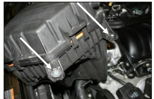
**6. Remove the two steel inserts, and grommets from the factory airbox.** Save these pieces, they will be reused in step #7.
