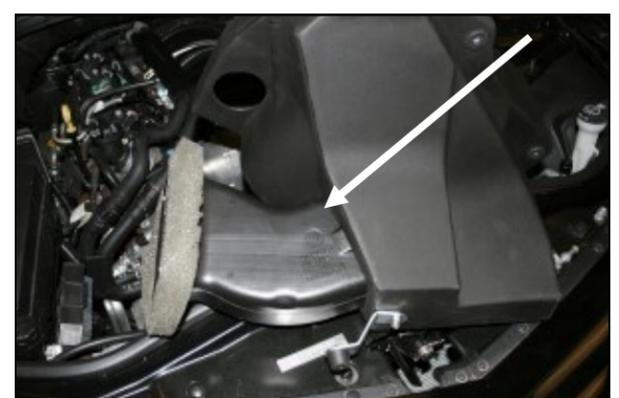
**9. Reinstall the factory scoop into the Airaid Cold Air Box.** It will snap into place.
