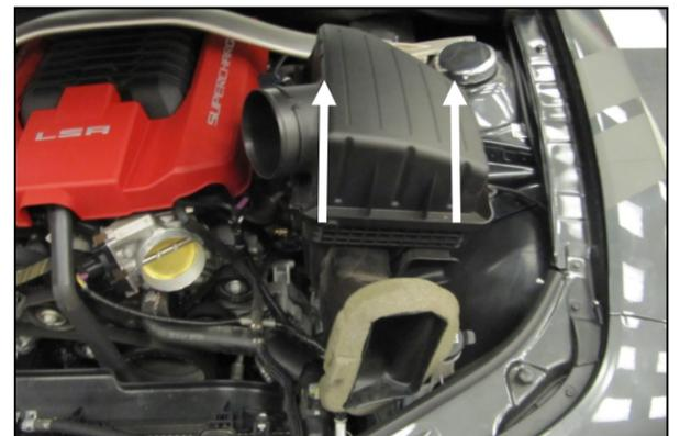
**3. Lift the airbox and scoop assembly straight up, and out of the vehicle.**
