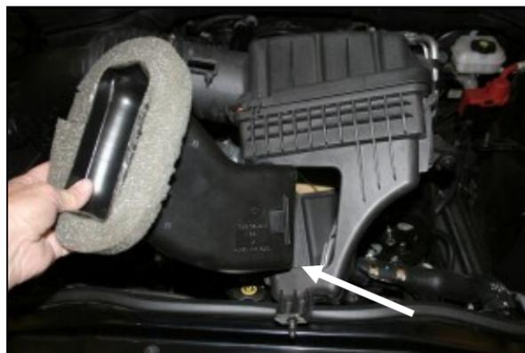
**5. Squeeze the sides of the factory intake scoop and remove it from the factory airbox.** It will be reused in step #9.
