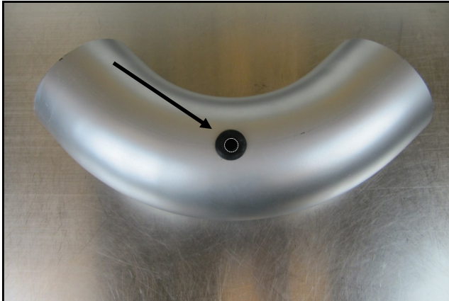
14. Insert the Grommet into the Airaid Intake Tube as shown.
