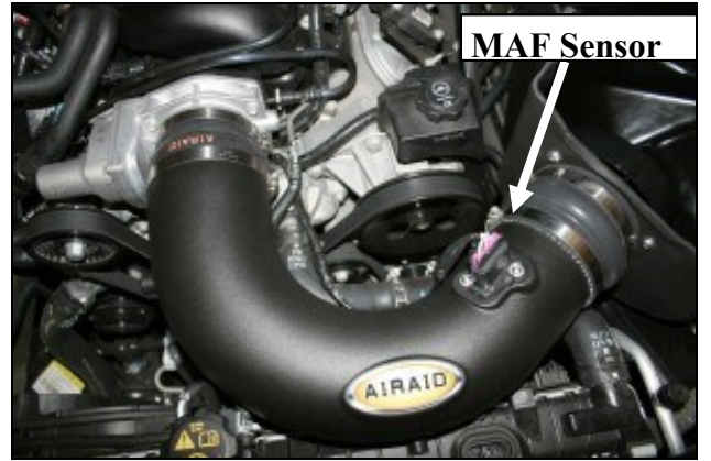
15. Install the Airaid Intake Tube (#2) into the hump hose first, and then into the reducing coupler. Adjust for fit, and tighten all four hose clamps. Next install the MAF sensor into the tube and secure it using two 8-32x3/8" button head screws (#16). Apply the Airaid Decal onto the Tube as shown.
