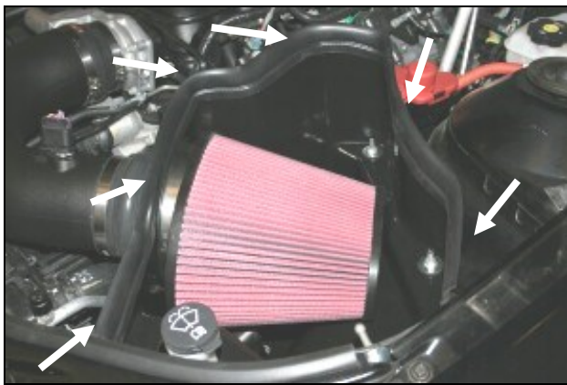
17. Install the Airaid Premium Filter onto the filter adapter and tighten the clamp. Next install the weather strip onto the top of the CAB. For ease of installation, start the front of the CAB near the radiator and work your way around towards the fender. Reinstall the engine beauty cover and oil fill cap.
