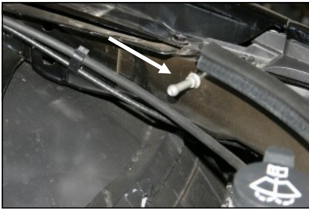
10. Using a 10mm wrench, remove and save the ground lug from the driver's side inner fender. It will be reused in step #12.
