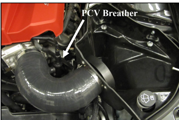
16. Install the Airaid Intake Tube assembly onto the Filter Adapter first, then onto the throttle body and tighten the clamps. Reconnect the PCV breather to the fitting and use the Speed Clamp (#22) secure the fitting in the tube. Reconnect the Mass Air Flow Sensor.
