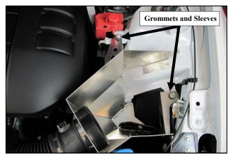
**11.** Install the Air Dam assembly into the inner fender area of the vehicle in the same manner as the OEM airbox. The grommets and sleeves are to be secured to the inner fender by re using the 6mm nuts that were removed in step Three.
