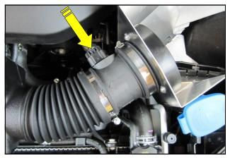
**13.** Check the positioning of the Mass Air Flow meter in relation to the wire harness. Readjust if necessary and tighten the clamps. Reconnect the Air Flow meter.
