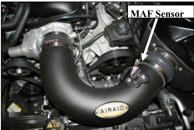
15. Install the Airaid Intake Tube (#2) into the hump hose first, and then into the reducing coupler. Adjust for fit, and tighten all four hose clamps. Next install the MAF sensor into the tube and secure it using two 8-32x3/8" button head screws (#16). Apply the Airaid Decal onto the Tube as shown.
