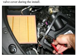
**4.**Turn the factory airbox lid over and locate the wire harness anchor. Using a pair of needle nose pillars, compress the ribs of the anchor and remove it. Remove the factory air filter and set it aside.
