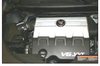
1. **Disconnect the negative battery cable.**Remove the oil fill cap and then lift up on the front of the engine cover to remove it from the vehicle. Replace the oil cap for now to make sure nothing falls into the
