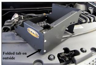
**5.** Join the two Airaid panels together with the folded tabs on the **outside**, using the four 6-32 screws (#15), #6 Flat washers (#14), and #6 Keps Nuts (#13). Apply the Airaid Decal onto the Panel as shown.
